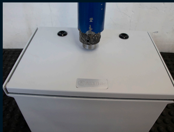
IK Testing *Photo taken in Allbro's Testing Lab
